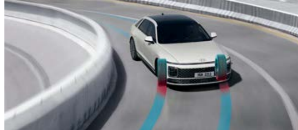
When the vehicle approaches a turn, the hybrid system regulates the vehicle's movement to execute torque vectoring while simultaneously maintaining the ideal level of tire grip for dynamic handling performance.
