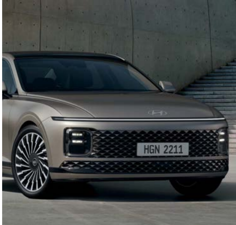
Parametric Pattern Grille / Horizontal LED lamp (Seamless Horizon Lamp) / Full LED Headlights (Projection Type)
