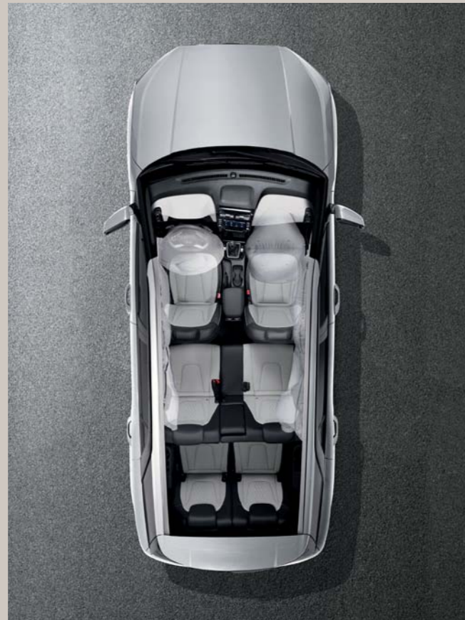
6-airbag system (Driver, Passenger, Side & Curtain) CRETA GRAND offers 6 airbags: the driver and front passenger get a pair of front airbags plus a pair of side airbags to protect the thorax and pelvic areas while left and right curtain airbags offer head protection for all cabin occupants.
