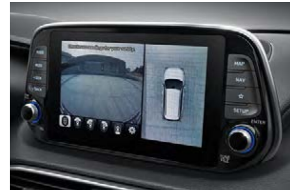
Hill-Start Assist Control (HAC) This system automatically holds the brakes to prevent the car from rolling back when starting from a hill. Surround View Monitor (SVM) A multi-camera system provides a 360-degree view around the vehicle to assist the driver in parking situations. * 8" touch screen may not be available in your country.
