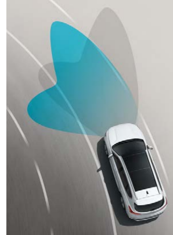
Low Beam Assist-Dynamic (LBA-D) The headlamps respond to the turn of the steering wheel and illuminate the part of the road the driver is turning towards.
