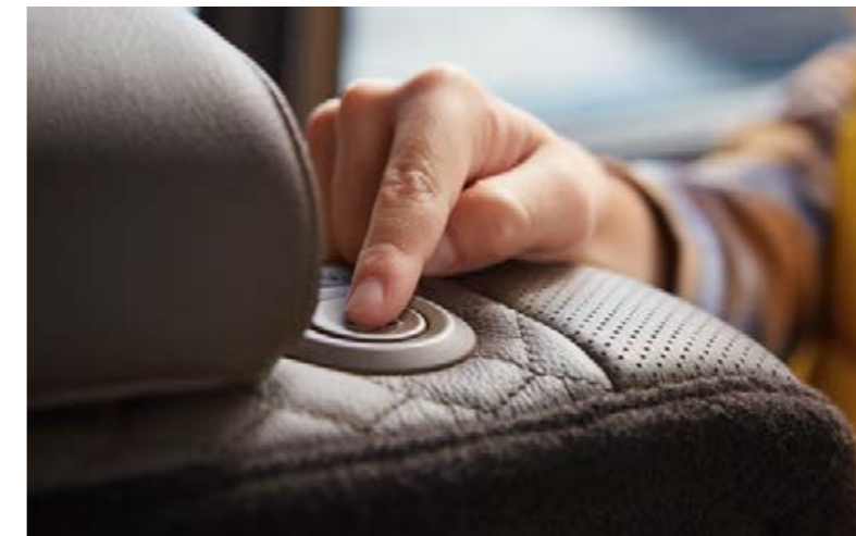
One-Touch Folding The one-touch folding feature allows you to fold the 2nd row seat easily by the push of a button.
