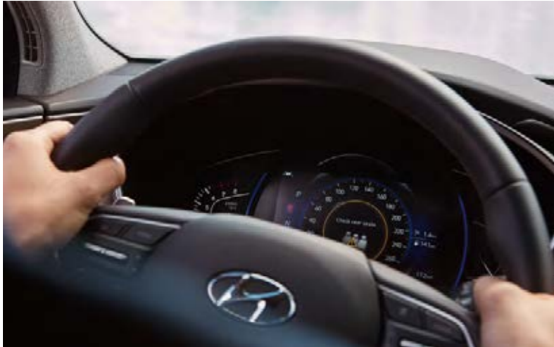
Rear Occupant Alert (First in class) The Rear Occupant Alert detects movement in the rear seats and reminds the driver there are rear occupants with an alert on the cluster. If the system detects movement after the driver has left the car and locked it, it sets off a sound alarm.
